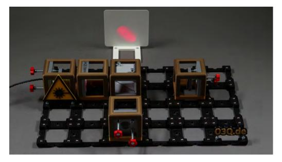
Figure 9. Low-Cost Michelson-Interferometer based on 3D-printing.
