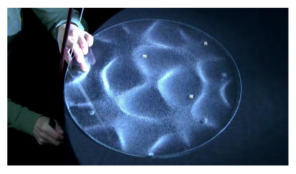
Figure 17. U2-5: Using Chladni sound figurs on a glass plate, nodal lines can be directly visualized.
